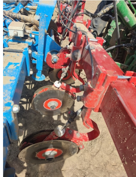
Figure 2 : the frame with disks for the banded fertilization system assembled on an existing single seed drill.
