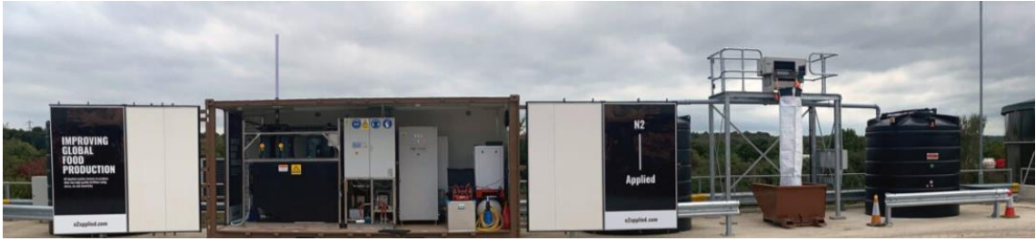
Figure 1 : The N2 unit at the University of Leeds farm showing from right to left: the raw slurry tank, separator, separated slurry tank, N2 unit and NEO storage tank.
