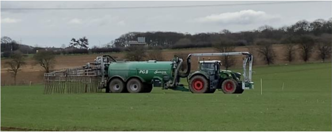
Figure 2 : Slurry application to winter wheat using dribble bars on the University of Leeds arable farm.
