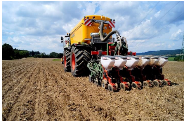
Figure 2: Strip tillage with slurry injection and planting.
